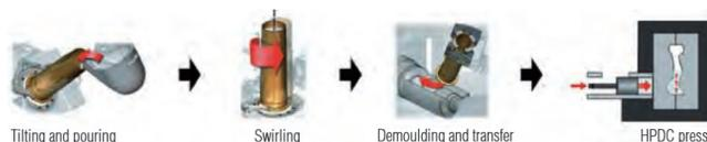
Fig. 1. SEED rheocasting method principle – phases [2]
