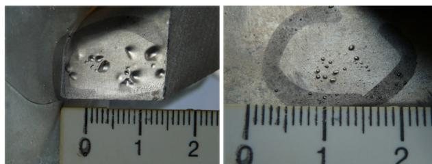
Fig. 2. Specific defects of casting appearing after heat treatment
