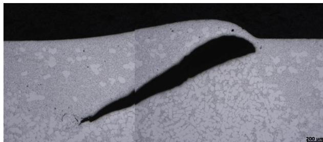
Fig. 5. Layer of eutectic structure covering the defect, 25x
