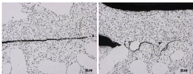
Fig. 6. Inner structure containing oxide films, 200x
