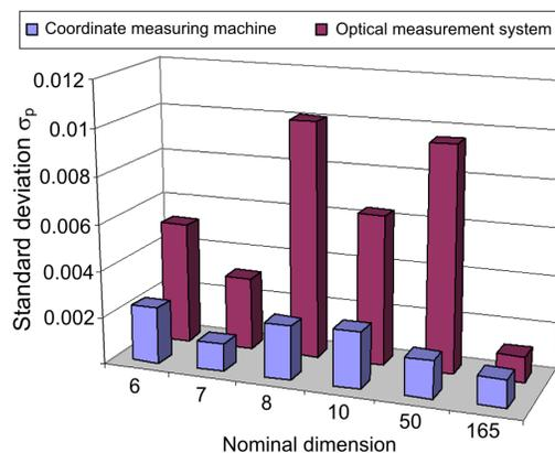
Fig. 4. The values of standard deviation of measurement repeatability error
