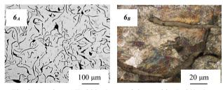
Fig. 3. Cast iron GJL-300:  $6_A$  – straight graphite IA3/4;  $6_B$  – pearlitic matrix, Sc = 0.98; A – unetched; B – etched with MilFe
