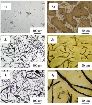
Fig. 1. Austenitic cast iron Ni-Mn-Cu:  $I_A$  – trace quantities of nodular graphite ID8;  $I_B$  – hypocutectic, chilled, Equ<sub>Ni</sub> = 19.4%, Sc = 0.55;  $2_A$  – straight flake graphite IA4 with some features indicating distribution type B;  $2_B$  – eutectic with flake graphite, Equ<sub>Ni</sub> = 18.7%, Sc = 1.06;  $3_A$  – primary graphite IC3;  $3_B$  – hypereutectic, Equ<sub>Ni</sub> = 17.1%, Sc = 1.48. A – unetched; B – etched with Mi1Fe
