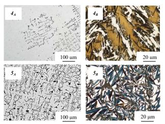
Fig. 2. Cast iron Ni-Mn-Cu:  $4_A$  – hypocutectic with small quantity of interdendritically distributed graphite colonies ID7;  $4_B$  – chilled, after partial austenite transformation, Equ<sub>Ni</sub> = 13.6%, Sc = 0.66;  $5_A$  – straight graphite IA5 with features indicating interdendritic distribution type E,  $5_B$  – martensite, Equ<sub>Ni</sub> = 11.6%, Sc = 0.98. A – unetched; B – etched with Mi1Fe
