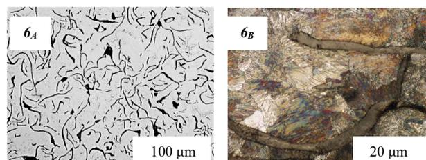
Fig. 3. Cast iron GJL-300:  $6_A$  – straight graphite IA3/4;  $6_B$  – pearlitic matrix,  $Sc = 0.98$ ;  $A$  – unetched;  $B$  – etched with Mi1Fe
