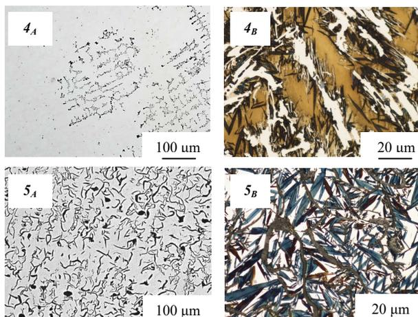
Fig. 2. Cast iron Ni-Mn-Cu:  $4_A$  – hypoeutectic with small quantity of inter-dendritically distributed graphite colonies ID7;  $4_B$  – chilled, after partial austenite transformation,  $Equ_{Ni} = 13.6\%$ ,  $Sc = 0.66$ ;  $5_A$  – straight graphite IA5 with features indicating interdendritic distribution type E,  $5_B$  – martensite,  $Equ_{Ni} = 11.6\%$ ,  $Sc = 0.98$ .  $A$  – unetched;  $B$  – etched with Mi1Fe
