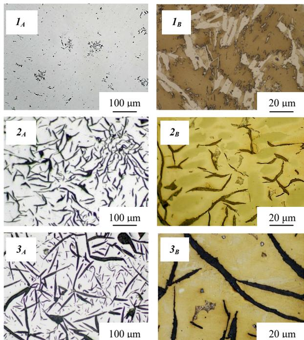
Fig. 1. Austenitic cast iron Ni-Mn-Cu:  $1_A$  – trace quantities of nodular graphite ID8;  $1_B$  – hypoeutectic, chilled,  $Equ_{Ni} = 19.4\%$ ,  $Sc = 0.55$ ;  $2_A$  – straight flake graphite IA4 with some features indicating distribution type B;  $2_B$  – eutectic with flake graphite,  $Equ_{Ni} = 18.7\%$ ,  $Sc = 1.06$ ;  $3_A$  – primary graphite IC3;  $3_B$  – hypereutectic,  $Equ_{Ni} = 17.1\%$ ,  $Sc = 1.48$ .  $A$  – unetched;  $B$  – etched with Mi1Fe
