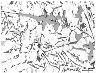
Fig. 4. The microstructure of silumin containing approximately 0.4% Cr and W obtained in the DTA sampler:  $\alpha$ ,  $\alpha$ +Al<sub>9</sub>Fe<sub>3</sub>Si<sub>2</sub>+ $\beta$ ,  $\alpha$ +Al<sub>2</sub>Cu+AlSiCuFeMgMnNi+ $\beta$
