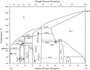
Fig. 1. Aluminum-chromium phase diagram [16]
