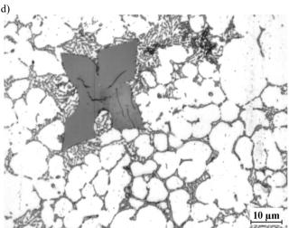
Fig. 5 (a-d). The microstructure of die casting made of the tested silumin containing Cr and W approximately: a-0.1%, b-0.2%, c-0.3% i d-0.4%:  $\alpha$ ,  $\alpha+Al_9Fe_3Si_2+\beta$ ,  $\alpha+Al_2Cu+AlSiCuFeMgMnNiCrW+\beta$
