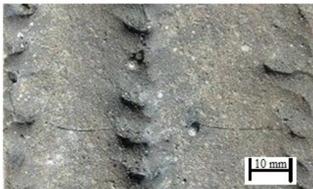
Fig. 16. Face inequalities by automatic welding.
