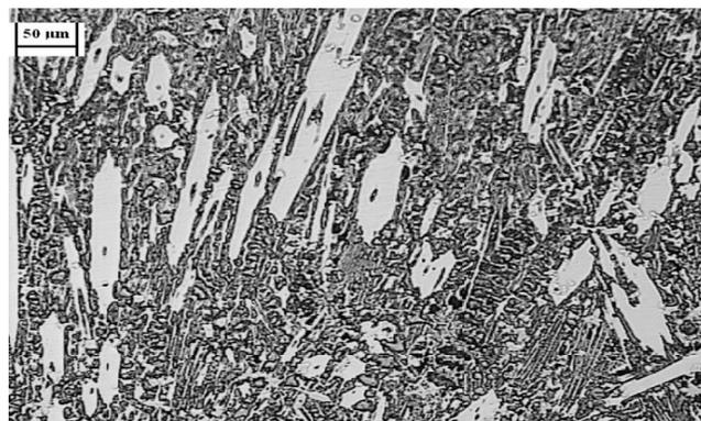
Fig. 2. Chromium carbides in the middle of surface layer
