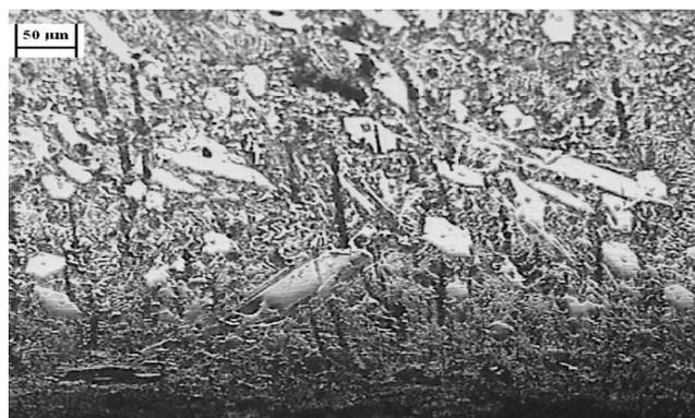
Fig. 3. Structure of material over the fusion line
