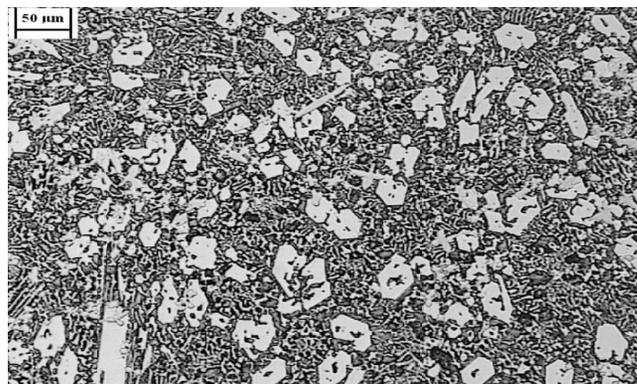
Fig. 1. Chromium carbides on the top of surface layer
