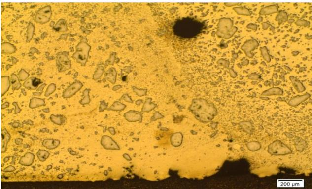
Fig. 5. Lack of fusion between the layer
