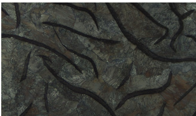
Fig. 7. The structure of cast iron samples no 1. 500x
