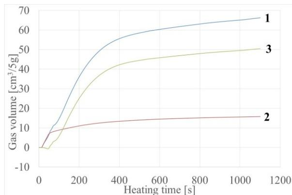
Fig. 5. Gases emissions from the moulding sand with resin: 1 – Total volume of gases flowing out of the flask, 2 – Volume increase of the air heated in the flask, 3 – Volume of gases originated from the moulding sand
