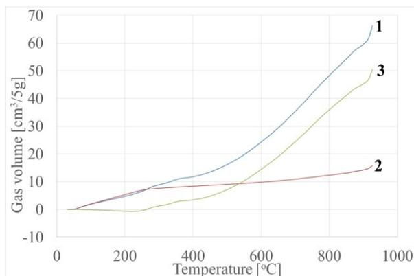
Fig. 6. Emission of gases in relation to the sample temperature: 1 – Total volume of gases flowing out from the flask, 2 – Volume increase of the air heated in the flask, 3 – Volume of gases originated from the moulding sand
