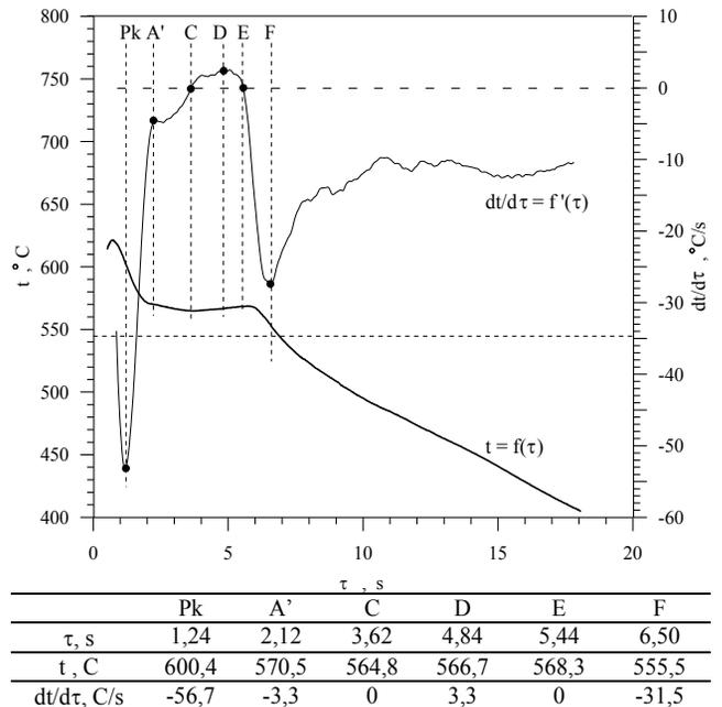
Fig. 4. TDA curves of solidification process of AlSi15 alloy with water mist cooling obtained by thermographic method
