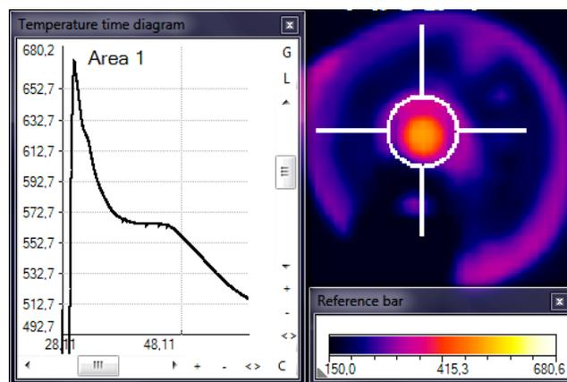
Fig. 2. Thermographic test results of Al-Si alloy during the solidification process
