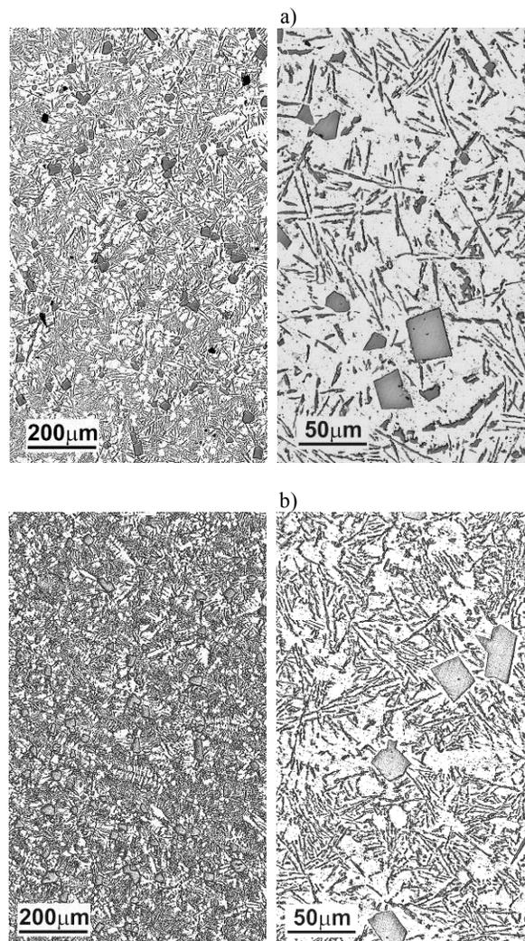
Fig. 7. Microstructure of AlSi15 alloy poured without cooling of probe (a) and with water mist cooling of metallic probe (b). Phase  $\beta$  (Si), lamellar eutectic  $\alpha+\beta$  (Al+Si)
