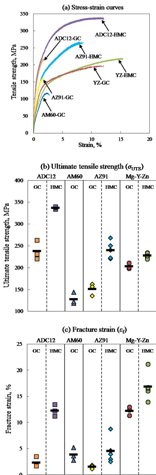
Fig. 3. Tensile properties of various cast samples, including YZ-GC and -HMC samples: (a) stress-strain curves, (b) ultimate tensile strength ( $\sigma_{UTS}$ ) and (c) fracture strain ( $\varepsilon_f$ )
