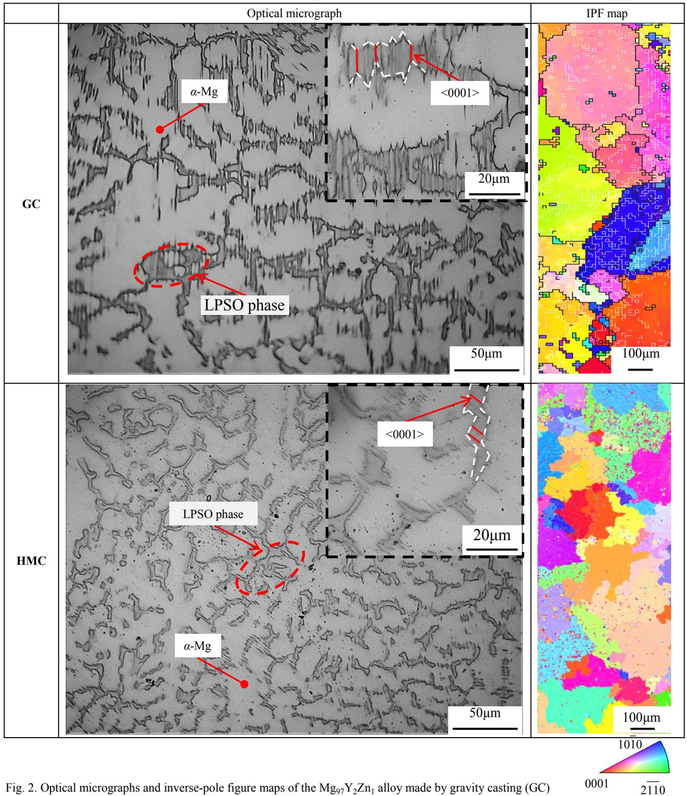
Fig. 2. Optical micrographs and inverse-pole figure maps of the  $Mg_{97}Y_2Zn_1$  alloy made by gravity casting (GC) and heated mold continuous casting (HMC)
