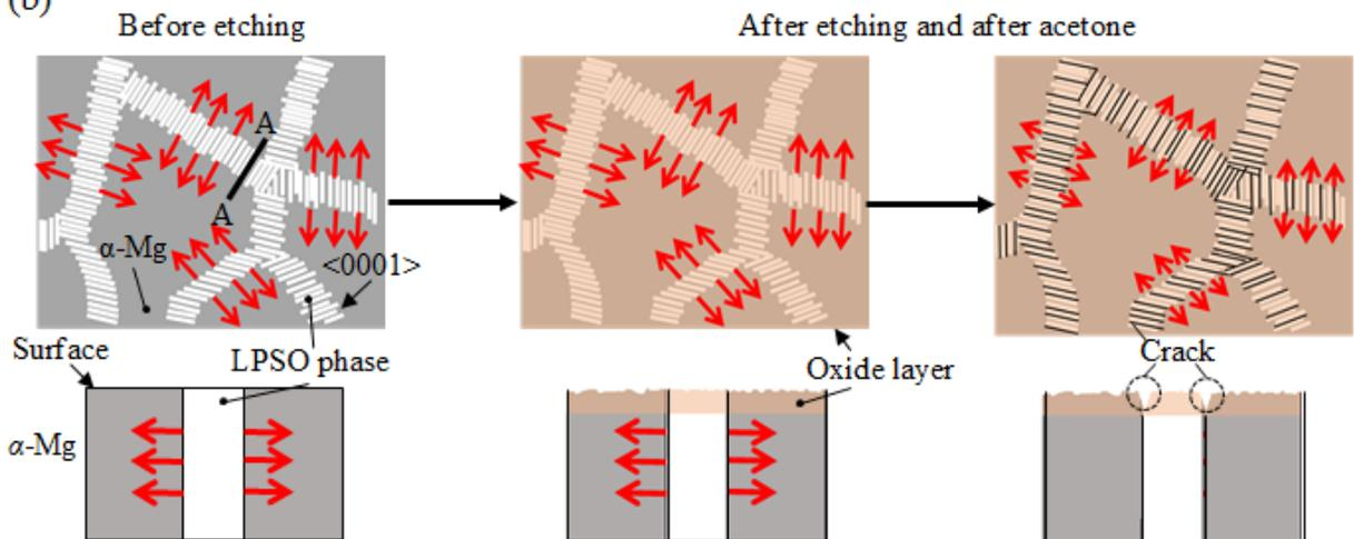
Fig. 8(a) SEM images of the YZ-HMC sample after the etching process, showing the residual stress areas indicated by different density of micro-cracks; Fig. 8(b) Schematic diagram showing the model of the revelation for the internal stress.
