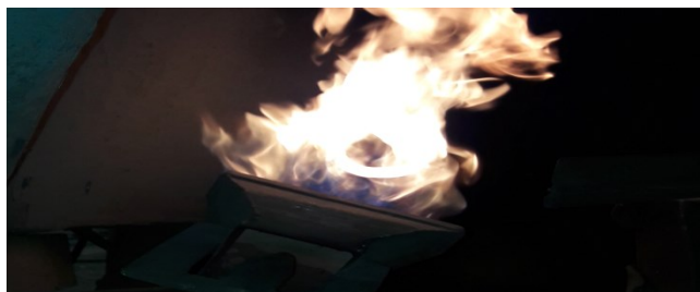
Fig. 5. Gas burner to preheating
