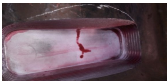
Fig. 4. The view of the surface checked by penetrant testing (PT)
