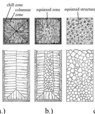
Fig. 1. Schematic illustration of three cast structures of metal: a.) pure metal, b.) solid-solution alloys, c.) structure obtained by using nucleating agents [1]
