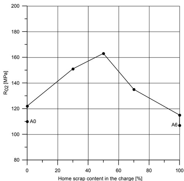
Fig. 2. The influence of the home scrap content in the charge on the yield strength of MgAl9Zn1 alloy castings
