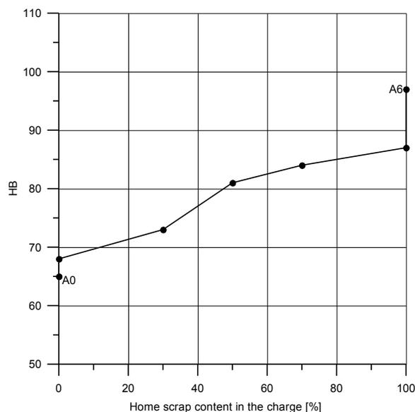
Fig. 4. The influence of the home scrap content in the charge on the hardness of MgAl9Zn1 alloy castings
