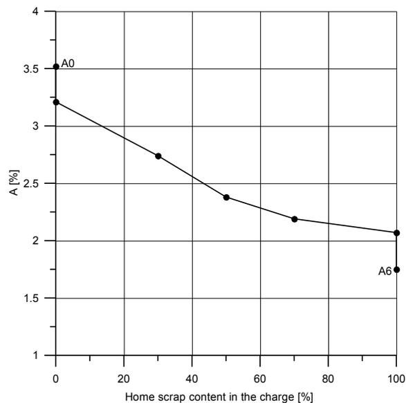
Fig. 3. The influence of the home scrap content in the charge on the unit elongation of MgAl9Zn1 alloy castings
