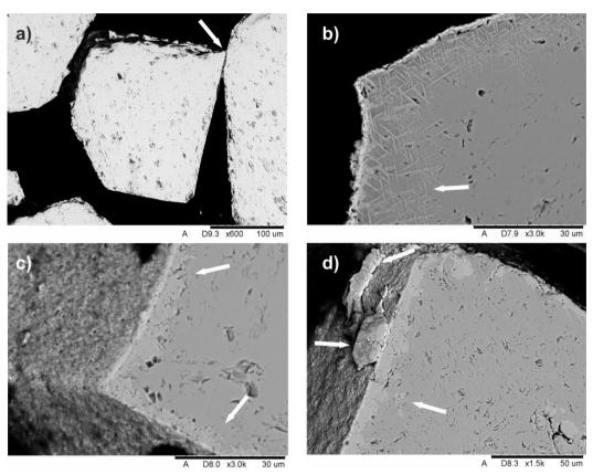
Fig. 4. Effect of heating temperature on chromite grain surfaces of moulding sand: a) 1000 °C, b) 1100 °C, and of pure sand: c) 1050 °C, d) 1100 °C. Sintered places on grain surface are visible in Fig. 4d.
