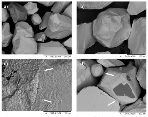
Fig. 3. Effect of heating temperature on grain surfaces of pure chromite sand: a)  $700\,^{\circ}$ C, b)  $800\,^{\circ}$ C, c)  $1050\,^{\circ}$ C, d)  $1100\,^{\circ}$ C. Linking bridges created after baking are visible in Fig. 3d.
