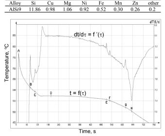
Fig. 2. Thermal analysis graph of EN AC 48000 alloy
