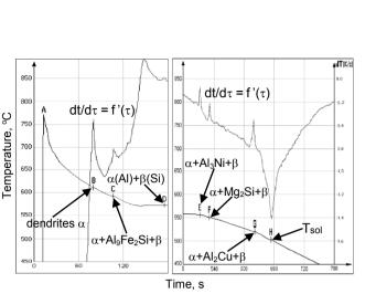
Fig. 3. Reduce scope of crystallization of EN AC 48000 alloy
