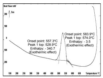
Fig. 5. DSC curve during cooling rate of EN AC 48000 alloy
