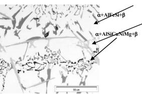
Fig. 6. Microstructure of EN AC 48000 cast alloy
