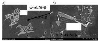
Fig. 8. Microstructure of EN AC 48000 alloy with visible eutectic mixtures containing: Al<sub>3</sub>Ni, Al<sub>2</sub>Cu and Al<sub>9</sub>Fe<sub>2</sub>Si phases
