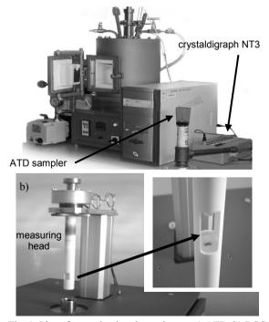
Fig. 1. Place for conducting thermal tests: a) ATD; b) DSC
