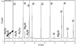
Fig. 7. Diffractograph of EN AC 48000 cast alloy
