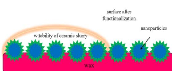
Fig. 5. Schematic diagram of functionalising of the wax pattern surface, used in the investment technology
