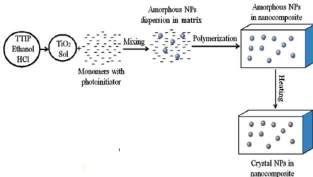
Fig. 1. Schematic of *in-situ* synthesis of hybrid materials [2]
