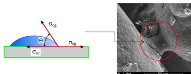
Fig. 7. Bridge joining the mineral matrix. 'Not coating' connection: binder/nanocomposite of the type: sodium silicate - MgO nanoparticles in propanol [11]
