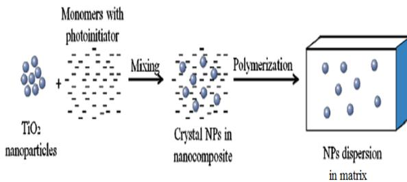
Fig. 2. Schematic of *ex-situ* synthesis of hybrid materials [2]
