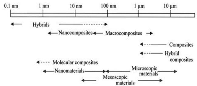
Fig. 3. Classification of the new generation materials, acc. to M. Nanko [3]
