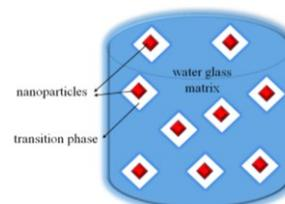
Fig. 6. Nanocomposite of the type: sodium silicate /metal oxides nanoparticles
