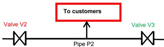
availability of water in the framework of this study is mainly dependent on the reliability of the pipe and of the valve (Fig. 4a).
