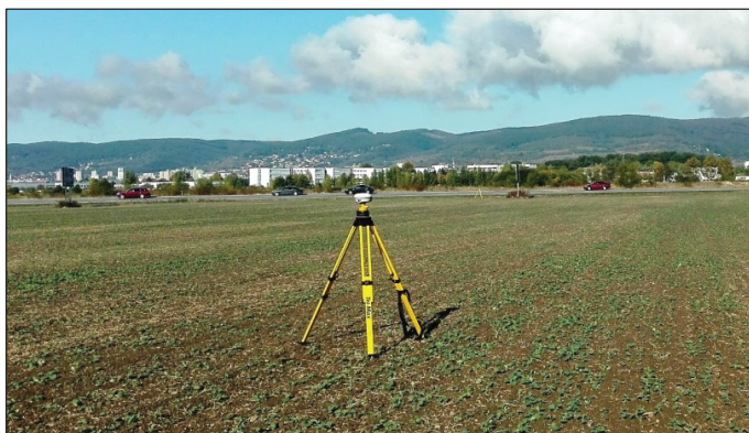
Fig. 3. Combined Trimble R8 Model 3 GNSS receiver setup in low-multipath environment during calibration measurement. Measurement took place near Bratislava – Vajnory, Slovakia on 7 October, 2016.
