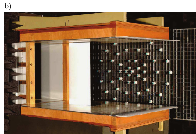
Fig. 2. Sketch of the NASA experimental setup (BROOKS et al. , 1989), (a) NRL's KAT wind tunnel test chamber instrumented with the microphones star array (b) (OERLEMANS, MIGLIORE, 2004; OERLEMANS, 2004).
