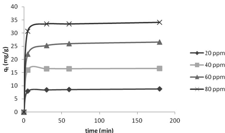
Fig. 2. Effect of initial concentration and time on the sorption of MB by immobilized *Yarrowia lipolytica* yeast (T= 25 °C, pH= 7, dosage= 0.1 g, agitation= 110 rpm)
