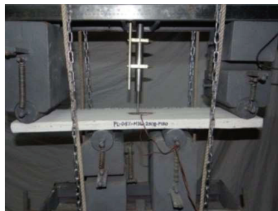
Fig. 2. Flexural Test Set-up (with test specimen)
