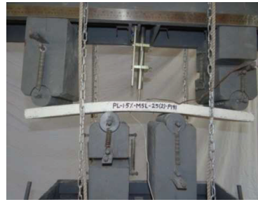
Fig. 8. Deflection Ductility of 5C
