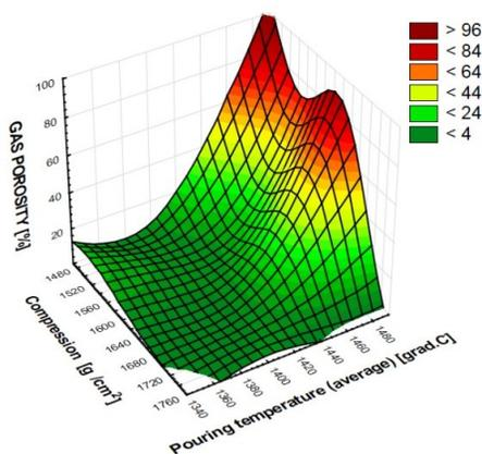
Fig. 4. Obtained visualization of the influence of the Compression and Pouring temperature parameter on the variation of percentage of Gas porosity defects revealed in castings
