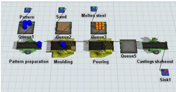
Fig. 3. Simplified model of steel casting foundry
