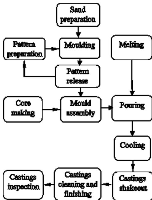
Fig. 2. Steel casting production process
