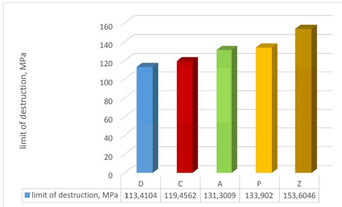
Fig. 8. The averaged results of the strength of the fresh rocks samples from different parts of the quarry
