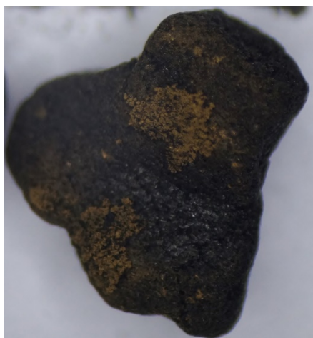
Fig. 5. Microscopic image of activated carbon after adsorption process
