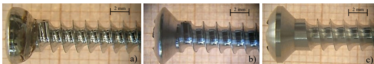
Fig. 2. Examples of screw surfaces from studied groups: a) I b), II c) III, stereoscopic microscope mag. 10× [30]
