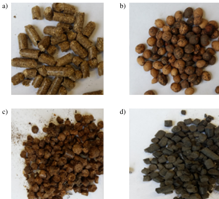
Fig. 3. Biomass types used in the study: a) wheat straw pellets, b) cherry stones, c) coffee husk pellets, d) sewage sludge pellets
