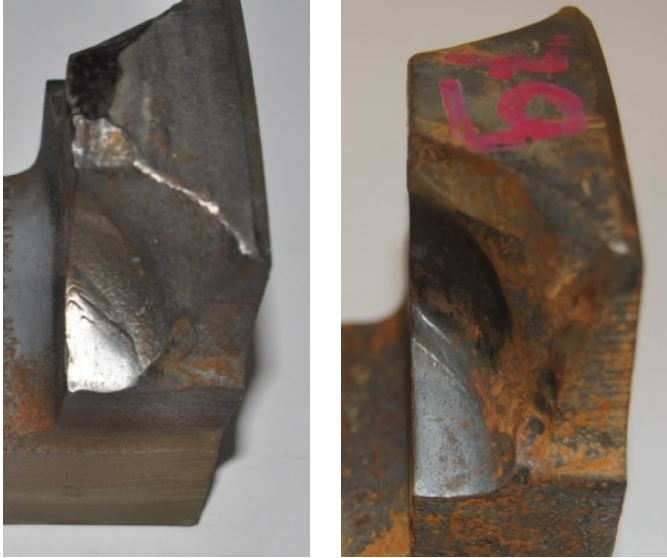
Fig. 11. Traces of abrasions on tooth surfaces of the test chain wheels made of ADI_360; A – the variant of wear involving quartz abrasive, B – the variant of wear involving quartz abrasive and salt solution
