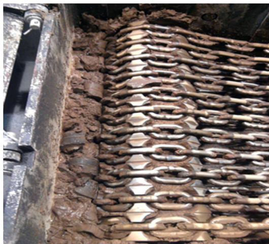
Fig. 6. A view of the test rig for wear tests filled with the abrasive mixture composed of quartz sand and water – at the final stage of the tribocorrosive wear tests
