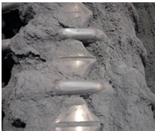
Fig. 4. A view of the chain wheels during the wear tests in the presence of the quartz abrasive
