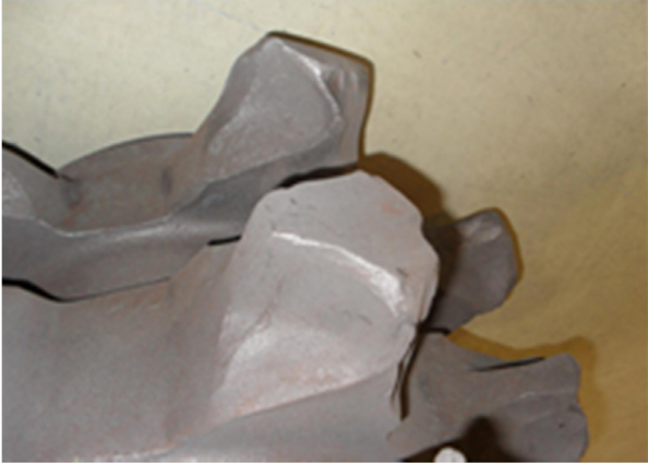
Fig. 1. An example view of tribocorrosive wear of a chain wheel in an armoured face conveyor
