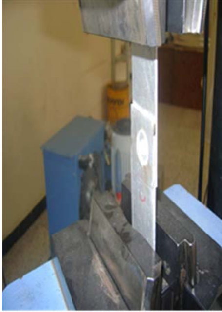
Fig. 5. An example of tensile shear test specimens
