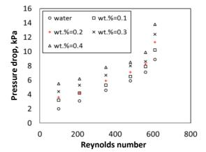
Fig. 4. Dependence of pressure drop on flow rate at different mass concentrations
