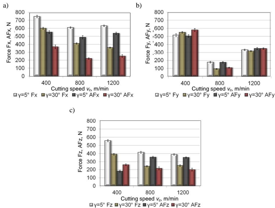
Fig. 2. The effect of change in cutting speed  $v_c$  on the value of cutting force components and their amplitudes during milling of AZ91HP magnesium alloy using tools of various rake angles: a)  $F_x, AF_x$ , b)  $F_y, AF_y$ , c)  $F_z, AF_z$
