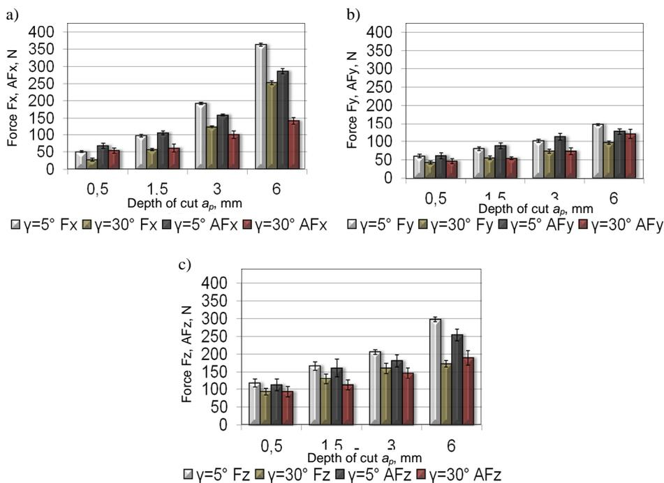
Fig. 4. The influence of change in depth of cut  $a_p$  (at  $f_z = 0.05$  mm/tooth) on cutting forces components and their amplitudes during milling of AZ91HP magnesium alloy using tools of various rake angles: a)  $F_x, AF_x$ , b)  $F_y, AF_y$ , c)  $F_z, AF_z$ ;  $f_z = 0.05$  mm/tooth,  $v_c = 800$  m/min
