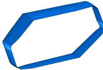
Fig. 2. Inverted joined wing isolated lifting surfaces model
