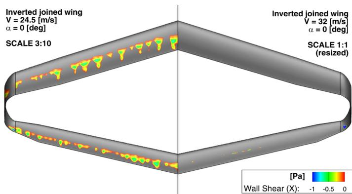
Fig. 12. Reversed flow regions for inverted joined wing lifting surfaces model (both scales compared)
