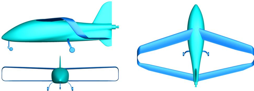
Fig. 1. Inverted joined wing complete airplane model
