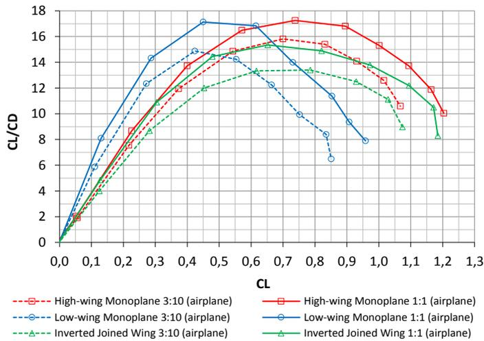
Fig. 10.  $CL/CD$  ratio vs.  $CL$  for all complete airplanes models
