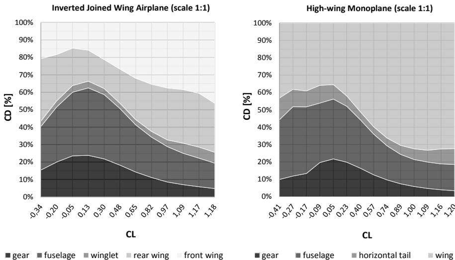
Fig. 15. The share of individual airframe parts in aerodynamic drag generation for inverted joined wing and ultralight high-wing monoplane – complete airplanes models (scale 1:1)
