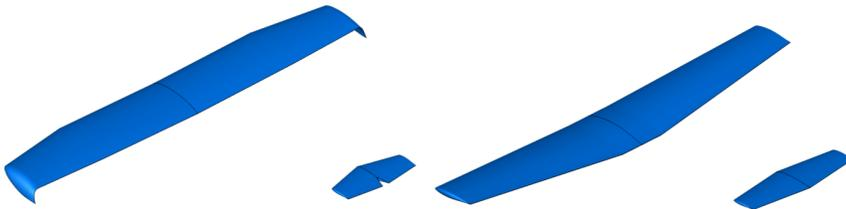
Fig. 3. First (high-wing) and second (low-wing) classical configuration isolated lifting surfaces model
