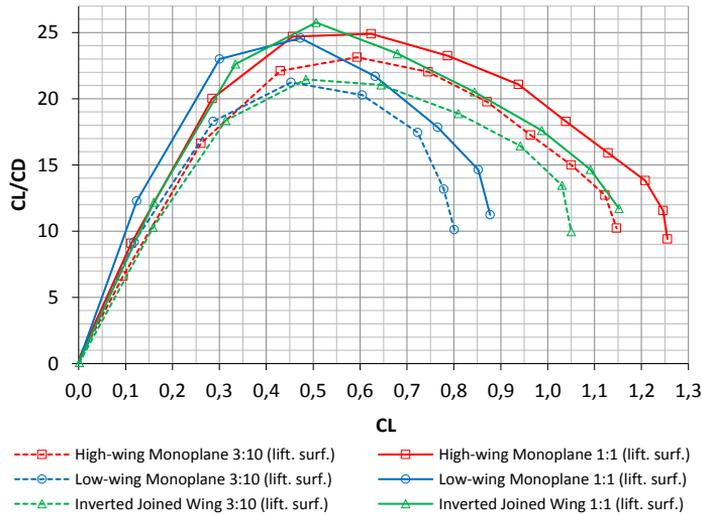
Fig. 8.  $CL/CD$  ratio vs.  $CL$  for all isolated lifting surfaces models
