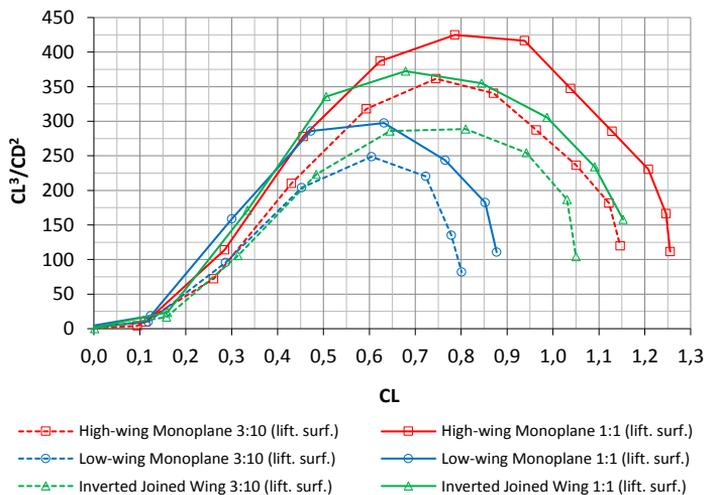
Fig. 9.  $CL^3/CD^2$  ratio vs.  $CL$  for all isolated lifting surfaces models
