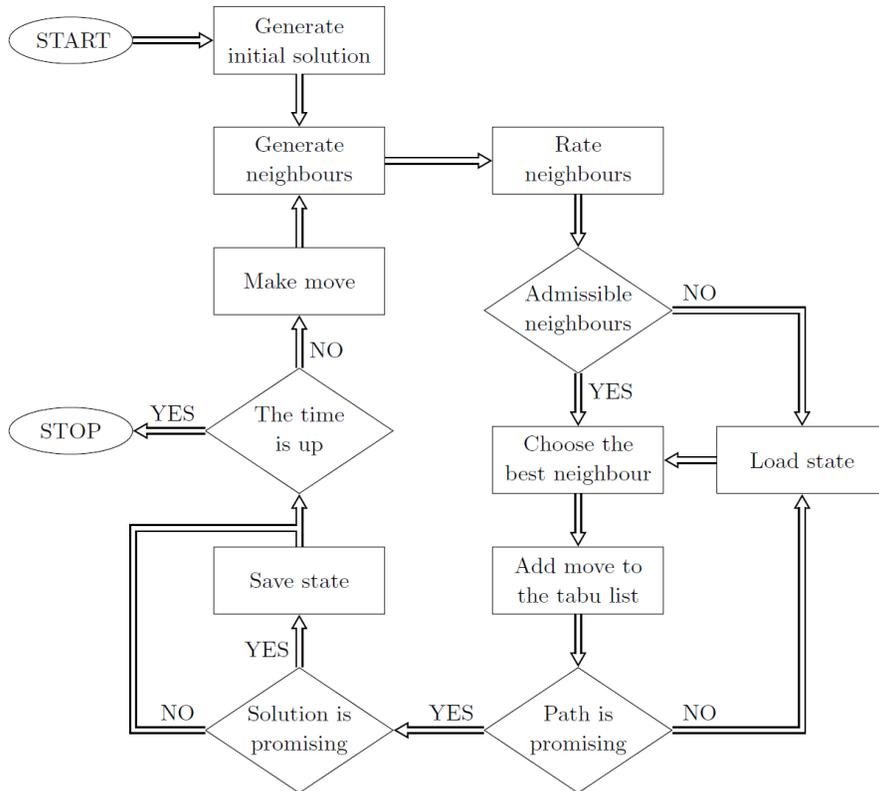
Figure 3: Schematic diagram of the Tabu Search algorithm.
