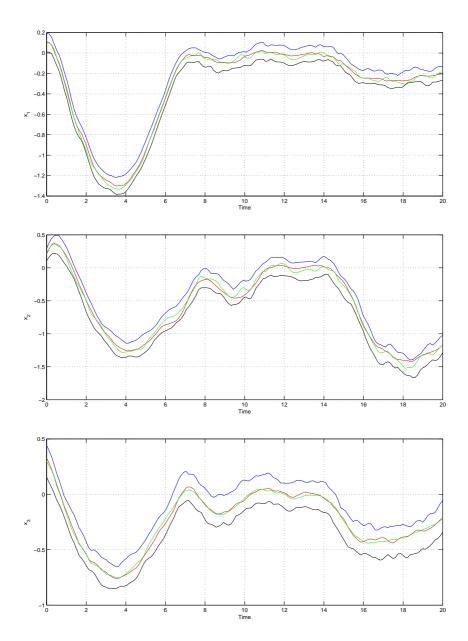
Figure 3: State  $x_1$ ,  $x_2$  and  $x_3$  bounds in blue and black lines with the Luenberger observer (green lines) and comparison with the real state (red line).
