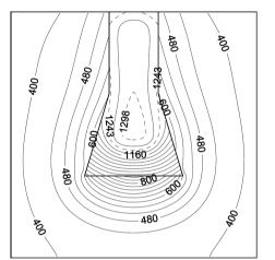
Fig. 5. Temperature distribution in the casting and the mold at t=100 s (unit: K)
