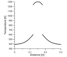
Fig. 3. Horizontal temperature distribution (y=0.2 m) at t=100 s
