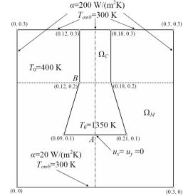
Fig. 2. Geometry of the casting and the mold with the boundary and initial conditions
