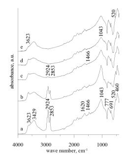
Fig. 4. IR spectra of the oil sand treated at temperature (a - 20°C, b - 70°C, c - 320°C, d - 450°C, e - 560°C)
