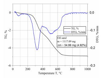
Fig. 2. TG/DTG curves for a sample of the oil sand
