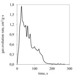
Fig. 6. The emission rate of gases from the oil sand
