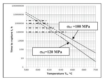
Fig. 1. Results of abridged creep tests of VM12 steel conducted at a temperature higher than the expected operating one and at constant stress level with different values ( $\sigma_{b1} = 100 \text{ MPa}$ ;  $\sigma_{b2} = 120 \text{ MPa}$ )
