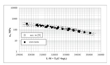
Fig. 2. Parametric average temporary creep strength curve in the form of relationship log  $\sigma_b = f(L-M)$  for VM12 martensitic steel under investigation. where: L-M is the Larson-Miller parameter; L-M =  $T_b(C + \log t_r)$ ,  $\sigma_b$  – test stress,  $t_r$  – time to rupture,  $T_b$  – test temperature in K, C = 37 – material constant
