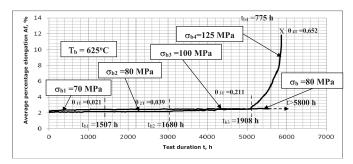
Fig. 7. Comparison of results of creep test with elongation measurement during testing in the form of creep curves  $\varepsilon = f(t)$  for various periodically changed levels of test stress  $\sigma_b$  at constant test temperature  $T_b = 625^{\circ}\text{C}$  to creep test conducted at constant temperature and stress parameters ( $\sigma_b = 80 \text{ MPa}$ ;  $T_b = 625^{\circ}\text{C}$ ) for VM12 steel
