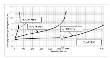
Fig. 3. Comparison of results of creep test with elongation measurement during testing in the form of creep curves  $\varepsilon = f(t)$  for different test stress levels  $\sigma b$  at constant test temperature  $T_b = 575^{\circ} C$  for VM12 steel
