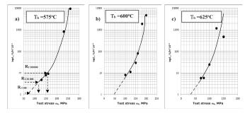
Fig. 9. Steady-state creep rate  $\dot{\epsilon}_s$  as a function of test stress level  $\sigma$  at constant test temperature Tb of VM12 steel: a) at  $T_b$ =575°C; b) at  $T_b$ =600°C; c) at  $T_b$ =625°C
