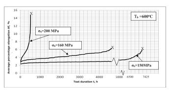
Fig. 4. Comparison of results of creep test with elongation measurement during testing in the form of creep curves  $\epsilon=f(t)$  for different test stress levels  $\sigma_b$  at constant test temperature  $T_b=600^{\circ}C$  for VM12 steel
