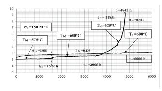
Fig. 8. Comparison of results of creep test with elongation measurement during testing in the form of creep curves  $\varepsilon = f(t)$  for different cyclically changed test temperature levels  $T_b$  at constant test stress level  $\sigma_b = 150 \text{MPa}$  to creep test conducted at constant temperature and stress parameters ( $\sigma_b = 150 \text{ MPa}$ ;  $T_b = 575^{\circ}\text{C}$ ) for VM12 steel
