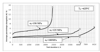
Fig. 5. Comparison of results of creep test with elongation measurement during testing in the form of creep curves  $\varepsilon = f(t)$  for different test stress levels  $\sigma_b$  at constant test temperature  $T_b = 625^{\circ}\text{C}$  for VM12 steel
