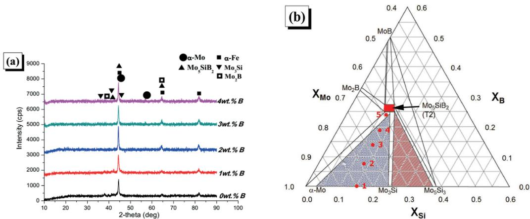
Fig. 6. (a) XRD graph of the Mo-Si-B coatings, (b) Mo-Si-B ternary phase diagram [15-18].
