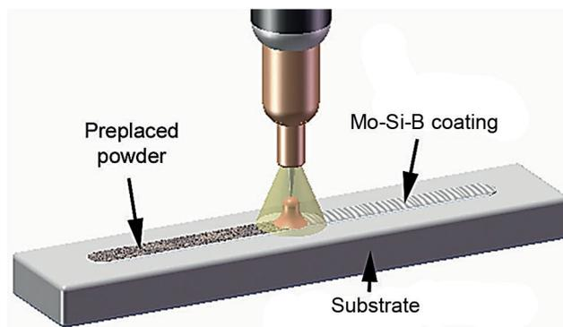
Fig. 1. Schematic diagram of the TIG process system
