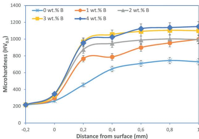
Fig. 7. Effect of boron content on Mo-Si-B coatings
