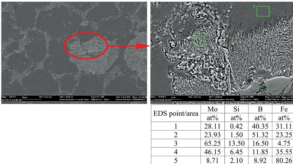
Fig. 5. SEM image and EDS analysis of the Mo-Si-3 wt.% B coating
