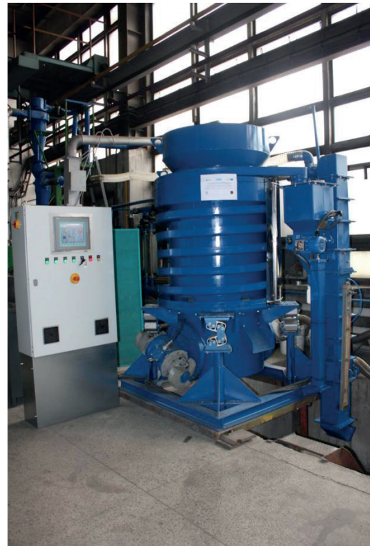
Fig. 1. Diagram of the prototypic REGMAS vibrating reclaimer: a) diagram: 1 – base frame, 2 – frame ledge, 3 – vertical brackets of oscillating supports, 4 – oscillating supports, 5 – device supporting structure plate, 6 – inner reclaimer column, 7 – cylindrical body, 8 – outer transport channel, 9 – channel (runner) cover, 10 – pneumatic cascade classifier, 11 – classifier support, 12 – auger feeder, 13 – feeder support, 14 – upper column segment, 15 – waste foundry sand container, 16 – grating for mould packages crushing 17 – central column segment, 18 – bottom column segment, 19 – upper flat sieve, 20 – central flat sieve, 21 – revision hole, 22 – bottom cone sieve, 23 – elastic sealing, 24 – fixing ring, 25 – covered channel, 26 – moulding sand buffer chamber, 27 – connection pipes with flanges, 28 – rotodynamic motors, b) view of reclaimer stand [8]
