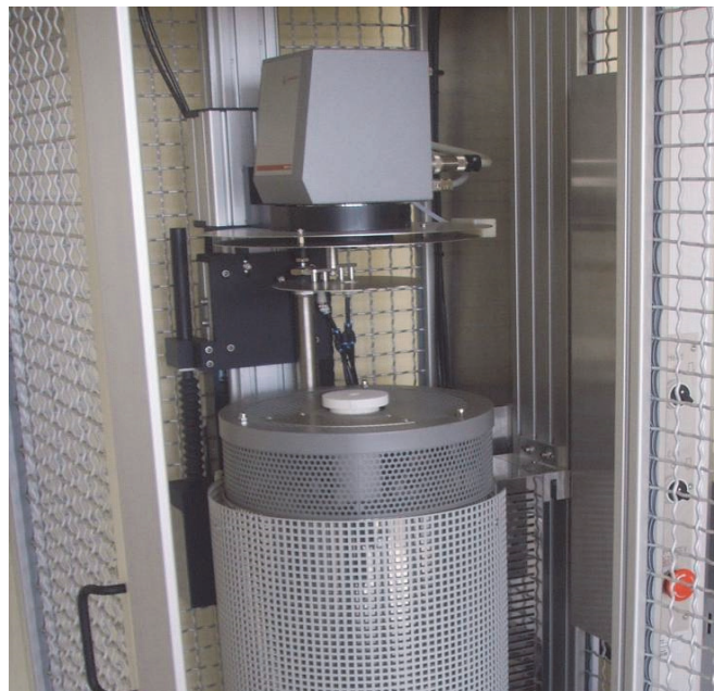
Fig. 2. Photograph of rotational viscometer used in investigations
