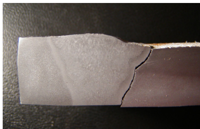
Fig. 2. The main crack from the pipeline's side extending through the HAZ – a cross section
