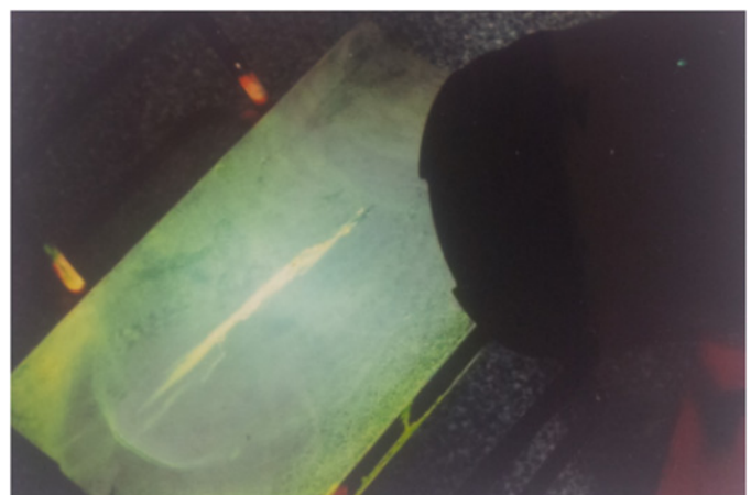
Fig. 1. Examples of indications obtained during penetrant testing: a) with the use of colour technique (the surface under testing is observed in natural or artificial white light), b) with the use of fluorescent technique (the surface is observed in UV radiation)
