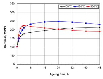
Fig. 6. Age hardening of cast Cu-3Ti alloy
