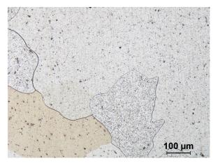
Fig. 7. Microstructure of cast Cu-3Ti alloy peak aged at 450°C for 24 h
