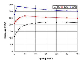
Fig. 14. Effect of prior cold drawing on hardness of Cu-3Ti alloy hot rolled, solution treated, cold drawn and aged at 450°C
