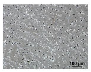
Fig. 4. Microstructure of homogenised Cu-3Ti alloy
