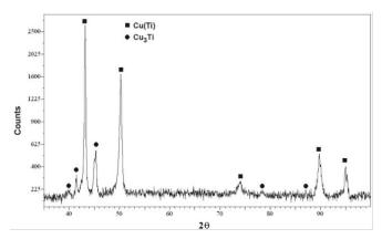
Fig. 3. XRD pattern of cast Cu-3Ti alloy
