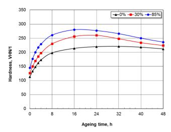
Fig. 11. Effect of cold drawing on hardness of Cu-3Ti alloy hot rolled, cold drawn, solution treated and aged at 450°C
