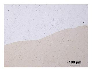
Fig. 5. Microstructure of Cu-3Ti alloy solution treated at 900°C for 2 h and quenched into water
