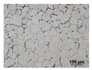
Fig. 9. Microstructure of hot rolled Cu-3Ti alloy
