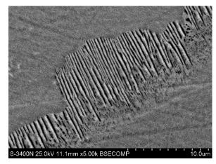
Fig. 8. Microstructure of cast Cu-3Ti alloy overaged at 450°C for 48 h
