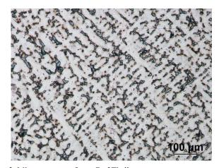
Fig. 2. Microstructure of cast Cu-3Ti alloy
