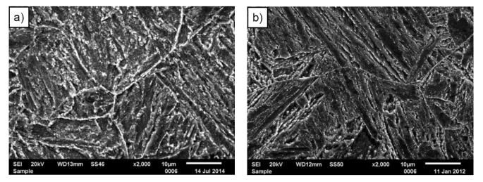
Fig. 1. Microstructure of the examined steels in the as-received state: a) P91; b) PB2, SEM
