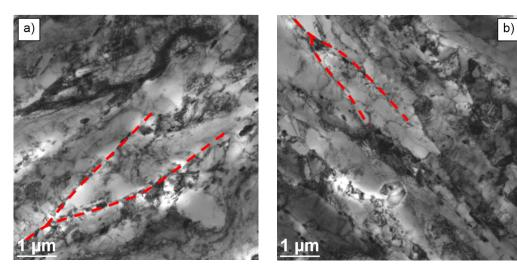
Fig. 10. Morphology of "Y" nodes in: a) P91 steel, b) PB2 steel, TEM
