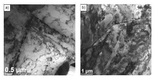
Fig. 12. Continuous grid of precipitates on the boundaries of prior austenite grain: a) P91 steel, b) PB2 steel, TEM
