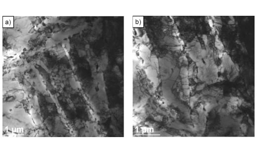
Fig. 11. Microstructure of the examined steels with visible wide and narrow laths of martensite: a) P91 steel, b) PB2 steel, TEM
