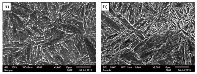
Fig. 7. Microstructure of the examined steels after ageing: a) P91; b) PB2, SEM
