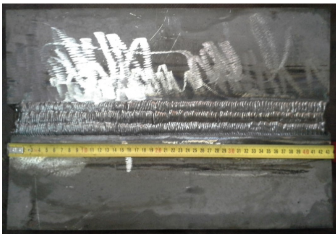
Fig. 3. A view of a sample welded joint from the weld's face
