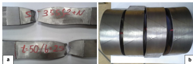
Fig. 4. A view of samples after testing: a) tensile test b) bending test (from the tensile side)
