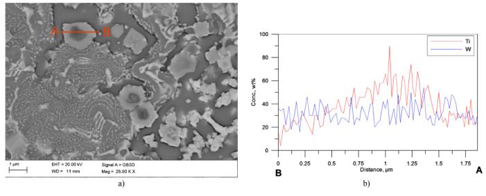
Fig. 10. a) representative BSE image showing the alloy matrix of the WTL produced under processing condition no WT3 (Table 2) and b) EDS line-scan analysis across the (Ti,W)C phase (profile taken along the line marked in Fig. 10a)
