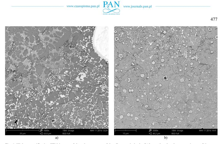
Fig. 4. Higher magnification SEM images of the microstructure of the alloy matrix in the SALs produced under processing conditions no: a) W1; b) WT1, Table 2
