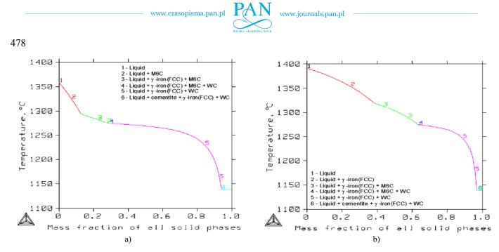
Fig. 6. Evolution of fraction solid versus temperature for solidification of the Fe-W-C alloy system at different composition calculated under Scheil conditions: a) Fe-30wt%W-2wt%C, a) Fe-20wt%W-1.25wt%C
