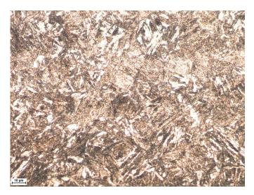
Fig. 1. Microstructure of the substrate material (ARMOX 500T)
