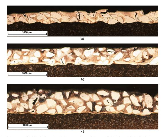
Fig. 2. Longitudinal macrographs of the WBs produced under processing conditions no: a) W1; b) WT1; c) WT3, Table 2
