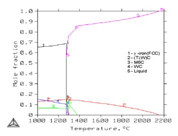
Fig. 9. Thermal stability of the phases in Fe-3wt%C-4wt%Ti-35wt%W alloy system
