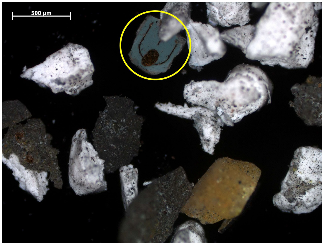
Fig. 3. LED chip in 106...1000 \mu\text{m} fraction (chip marked with circle)
