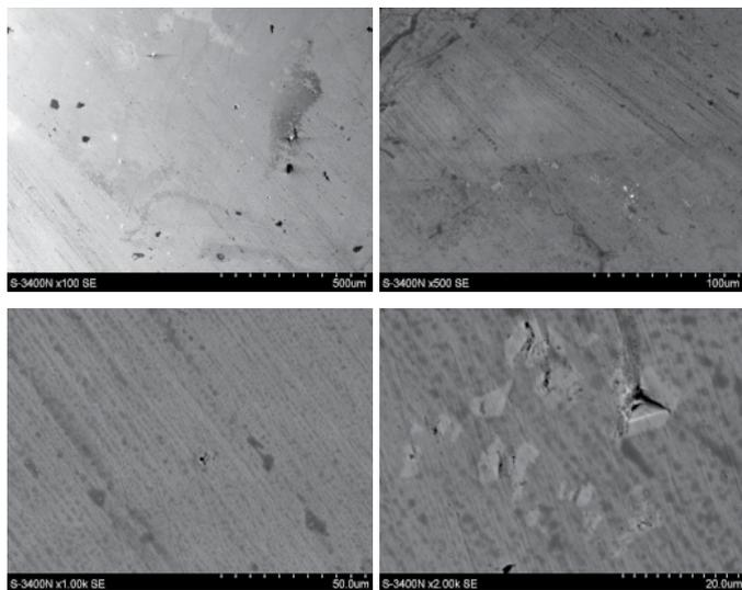
Fig. 2. Morphology of corrosion damage to the base material of the Inconel 625
