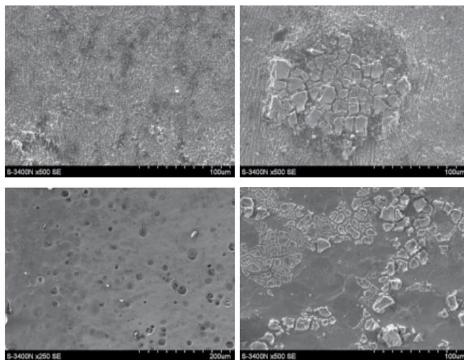
Fig. 4. Morphology of corrosion damage in Inconel 625 weld
