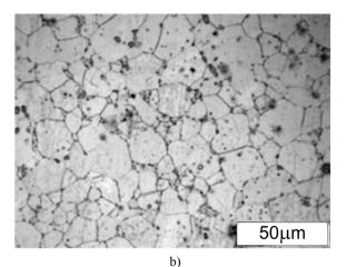
Fig. 2. Microstructure of the casting process and heat treatment: a) AZ61, b) WE43
