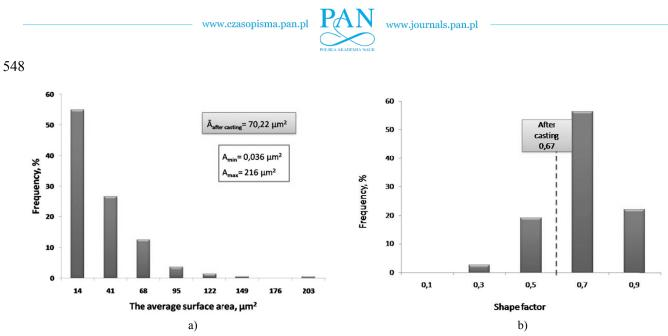
Fig. 5. The average surface area, b) the shape index grain size of the alloy AZ61 after the extrusion KOBO method
