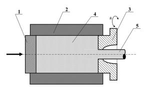
Fig. 1. Diagram of direct extrusion: 1 – punch, 2 – container, 3 – cyclic rotated die with grooves on face area surface, 4 – extruded material, 5 – charge/product [2]
