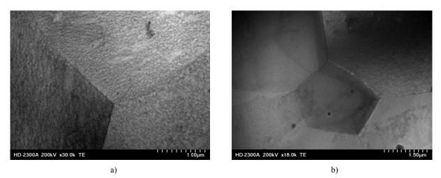
Fig. 6. Substructure of alloys after extrusion KOBO method: a) AZ61, b) WE43
