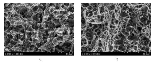
Fig. 9. Results of fractographic tests of sample fractures in alloy WE43 after static tension test in room temperature after: a) classic extrusion, b) extrusion KOBO method
