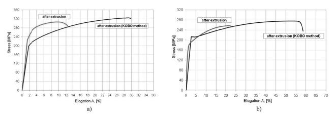
Fig. 7. Strain curvefor the investigated at room temperature: a) AZ61, b) WE43
