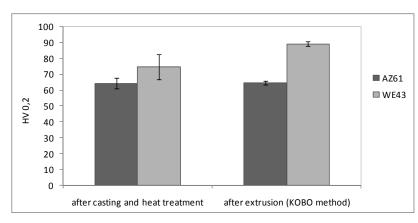
Fig. 10. Results of micro-hardness measurements for alloys AZ61, WE43 in initial state and after extrusion KOBO method
