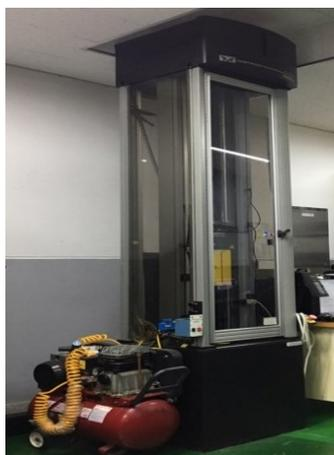
Fig. 2. Impact test device Dynatup 9250 HV
